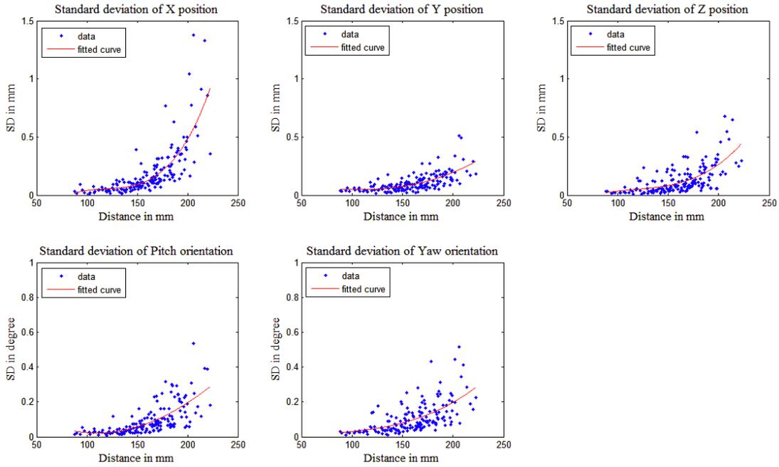
environment. The horizontal axis represents the distance between the sensor and the middle point of the transmitter coils, and the vertical axis represents the standard deviations.
