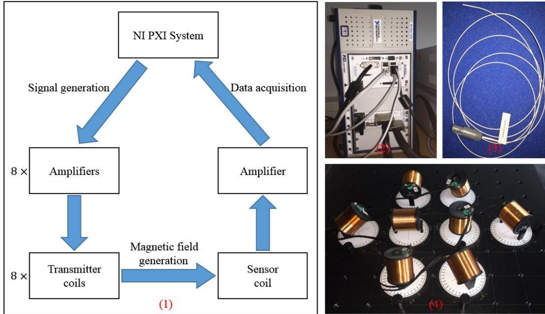
Figure 1. The experimental setup of the electromagnetic tracking system: (1) system block diagram, (2) NI PXI system, (3) NDI Aurora 5-DOF catheter, (4) Transmitter coils.
