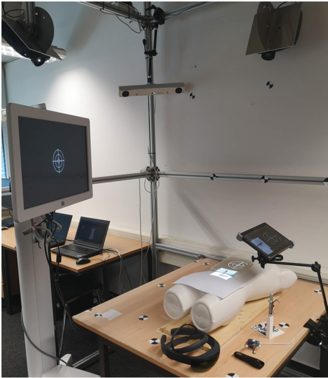
Fig. 3. Study apparatus. VST tablet computer, OST HMD, projector-camera-system and monitor were used to display navigation aids. An optical tracking camera was used to obtain needle position data and for phantom registration. Only the projector opposite from the participant was used (top left image corner).
