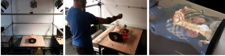
**Fig. 2.** The experimental setup. Projectors mounted above a table superimpose a torso phantom with a medical volume data set.
