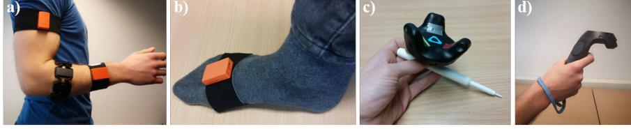
**Fig. 1.** Apparatus of implemented interaction techniques. a) Hand gestures. b) Foot gestures. c) Surgical instrument. d) Controller.
