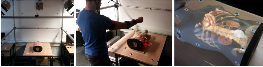
**Fig. 2.** The experimental setup. Projectors mounted above a table superimpose a torso phantom with a medical volume data set.
