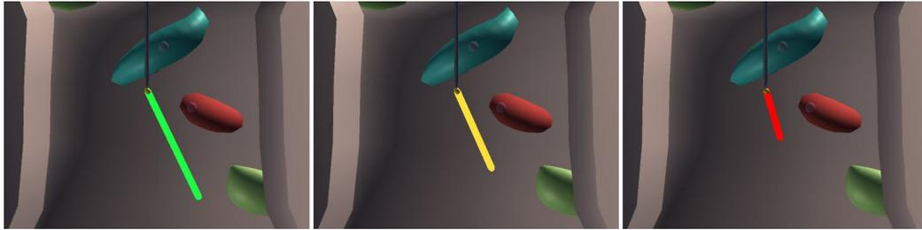
Figure 2. Side-looking radar. A radar rotates around an instrument at an adaptable angle. It ends when a collision with an object is detected. The color of the line is determined by the distance to the detected collision.
