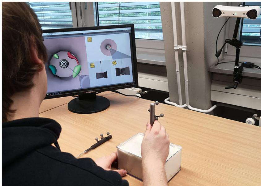
Video 1. Experimental Setup. A user is navigating a tracked instrument inside a virtual cavity within a curd filled phantom. A Monitor shows the developed navigation environment. Different visualization concepts are presented in the video: <http://dx.doi.org/doi.number.goes.here>
