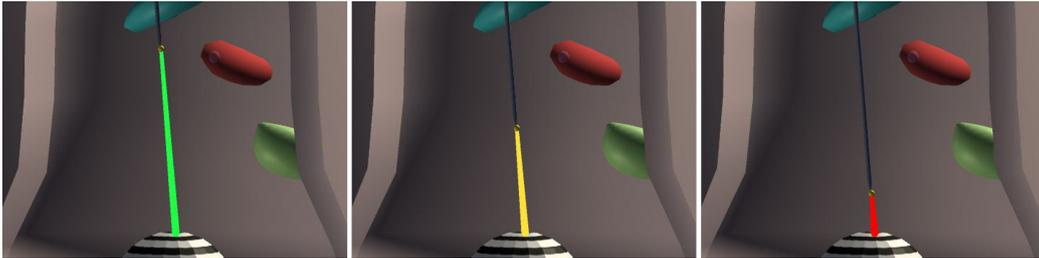
Figure 1. Pointer Ray. An instrument is virtually extended by a ray pointing at potential collisions along the trajectory. The distance to detected objects is encoded by the line color.
