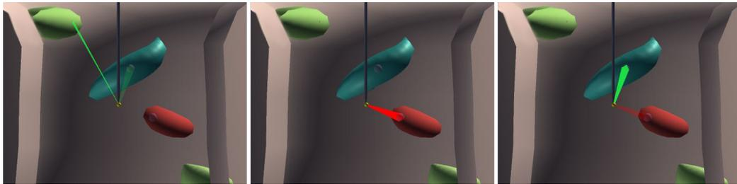
Figure 3. Virtual lighthouses. Each lighthouse emits a color-coded signal pointed towards an instrument (green and red lines). Displayed rays appear one after another and then slowly fade out.
