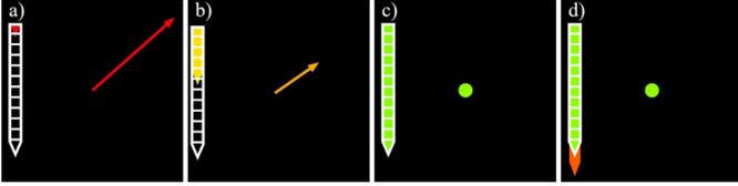
Fig. 3. Arrow Concept. An arrow glyph indicates angular deviations and a progress bar represents insertion depth information. The arrow is pointed towards the planned insertion trajectory. Its length represents angular deviations. From left to right the insertion angle is steadily improved and the needle gets further inserted. (d) shows a needle that was inserted too far. Colors are mapped to accuracy levels.
