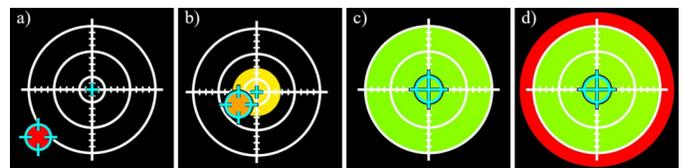
Fig. 2. Crosshairs Concept. The needle handle is projected onto a crosshairs grid (blue). For correct needle orientation, the marker has to align with the crosshairs' center. The grid is steadily filled to encode insertion depth information. From left to right the insertion angle is steadily improved and the needle is inserted further. (d) shows a needle that was inserted too far. Colors are mapped to accuracy levels.
