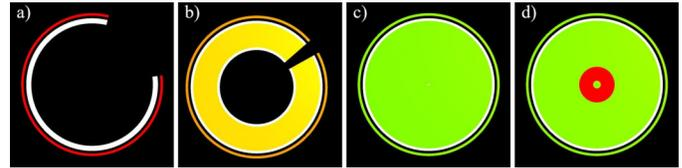
Fig. 1. Circle Concept. Concentric circular arcs encode insertion depth and angular accuracies. Arcs are opened towards planned insertion trajectory. Opening angles represent angular deviations and arc diameters encode insertion depth information. From left to right, the insertion angle is steadily improved and the needle is inserted further. (d) shows a needle that was inserted too far. Colors are mapped to accuracy levels.
