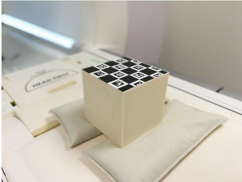
Figure 4: Calibration body filled with candle wax for MRI imaging and with a ChArUco board attached to estimate the phantom's pose in camera coordinates.
