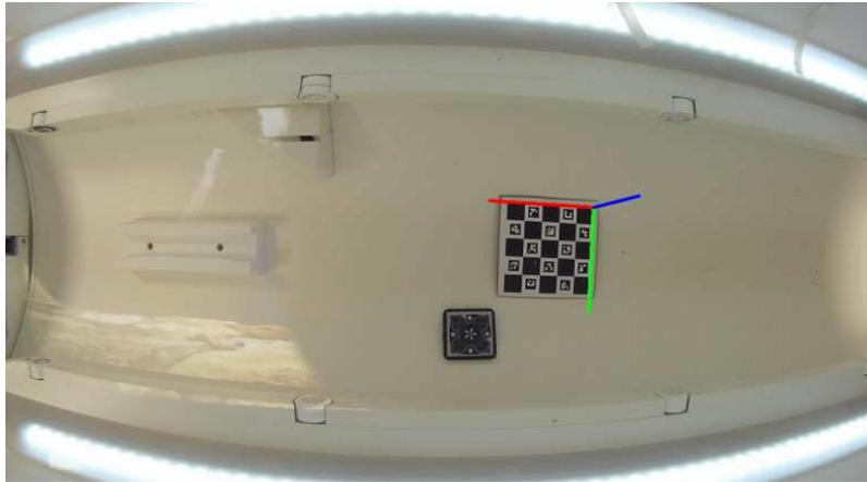
Figure 3: Estimation of the fixed ChArUco marker pose for registration of the MRI coordinate system with the camera coordinate system.
