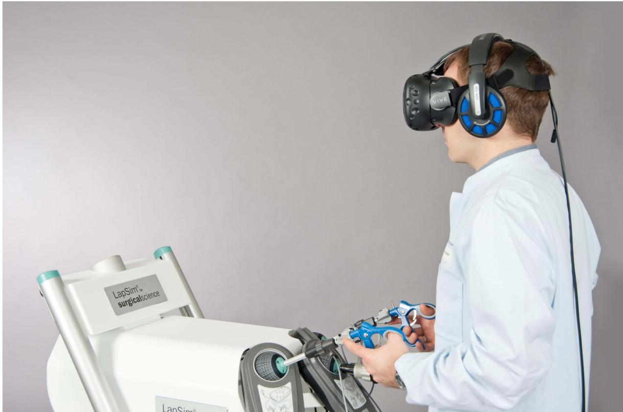
**Fig. 1:** Custom IVR setup with LapSim Simulator with the 4D joysticks (Simball, G-coder Systems, Sweden); the goggles are the HTC Vive (HMD); and the headphones provide sound. A conventional monitor is not needed in this setup.
