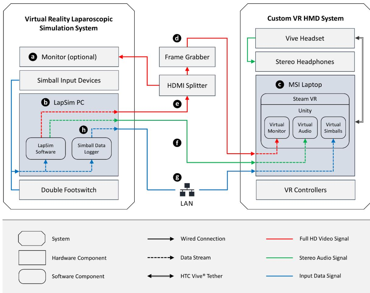
**Fig. 2:** Component diagram of the VR laparoscopy simulation system and our customized VR HMD system. a: conventional 2D screen, b: surgical simulator, c: VR-ready MSI laptop, d: HDMI to USB frame grabber, e: HDMI signal splitter, f: stereo audio cable, g: local network connection (LAN), h: Simball data logger auxiliary program.
