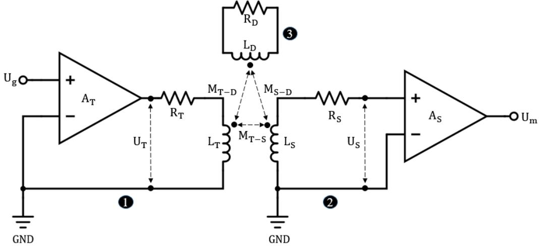
Fig. 2. The RL circuit model of (1) one out of the eight transmitter coil circuits, (2) the sensor coil circuit and (3) the circuit of the conductive distorter.
