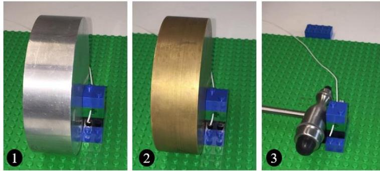
Fig. 7. Time constant measurement of metal distorters: (1) an aluminum disk with a diameter of 10 cm and thickness of 3 cm, (2) a brass disk with a diameter of 10 cm and thickness of 3 cm, (3) a neurological reflex hammer.
