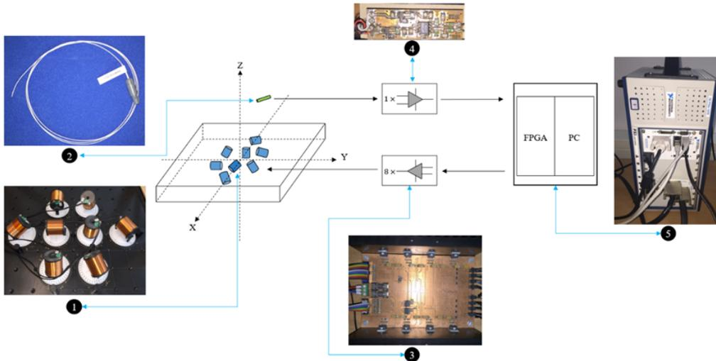
Fig. 1. Schematic diagram of our ETMS configuration: (1) eight self-developed transmitter coils, (2) sensor coil, (3) eight current-feedback amplifiers for signal generation, (4) pre-amplifier for the measured signals, and (5) the control and signal generation and data acquisition system comprising an FPGA and a PC.
