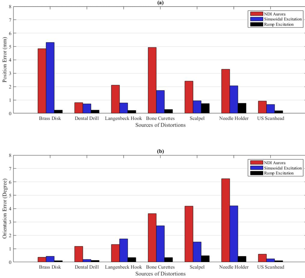
Fig. 14. Sensor pose's error resulting from different sources of distortion for our experimental setup applying ramp/ sinusoidal excitations and the commercial system: (a) sensor position error, (b) sensor orientation error.
