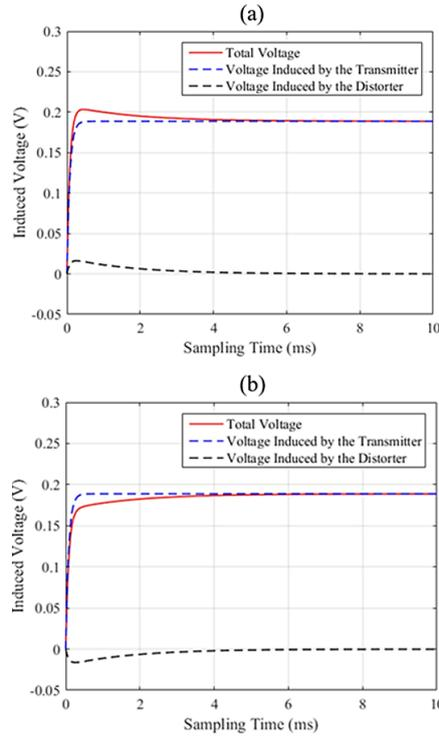
Fig. 3. An example of the simulated voltage measurement with a conductive distorter nearby the sensor coil: (a) additive conductive distortion, (b) subtractive conductive distortion between sensor and distorter.
