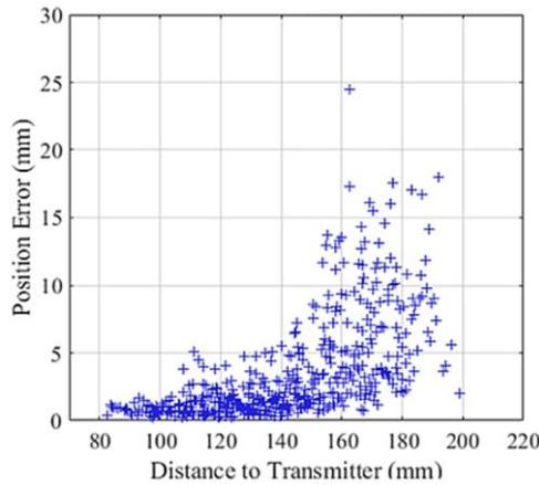
Fig. 12. Sensor position error in the test volume with distance between the sensor and the center of the transmitter coils array of up to 200 mm.
