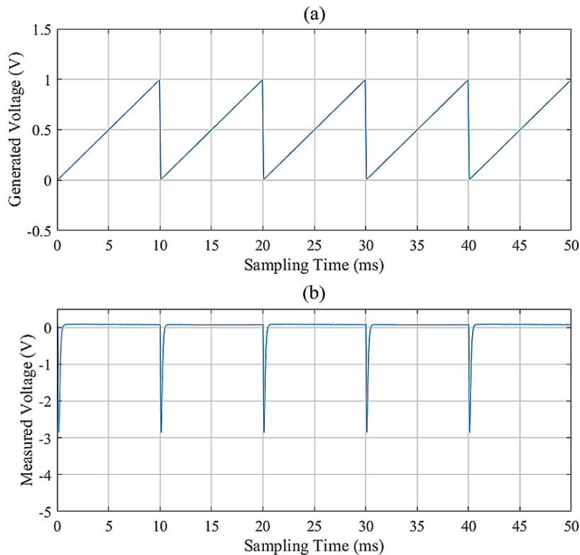
Fig. 5. Generated and measured voltages: (a) voltage generated by DAC and (b) an example of the voltage induced by one of the eight transmitter coils measured by ADC.
