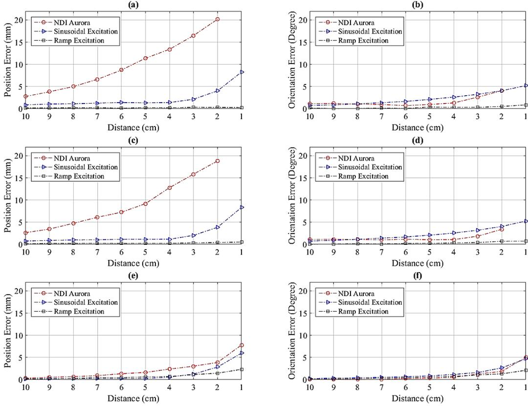
Fig. 13. Sensor pose error due to conductive distorters placed at different distances to the sensor coil: (a) position error due to an aluminum disk, (b) orientation error due to an aluminum disk, (c) position error due to a brass disk, (d) orientation error due to a brass disk, (e) position error due to a reflex hammer, and (f) orientation error due to a reflex hammer.
