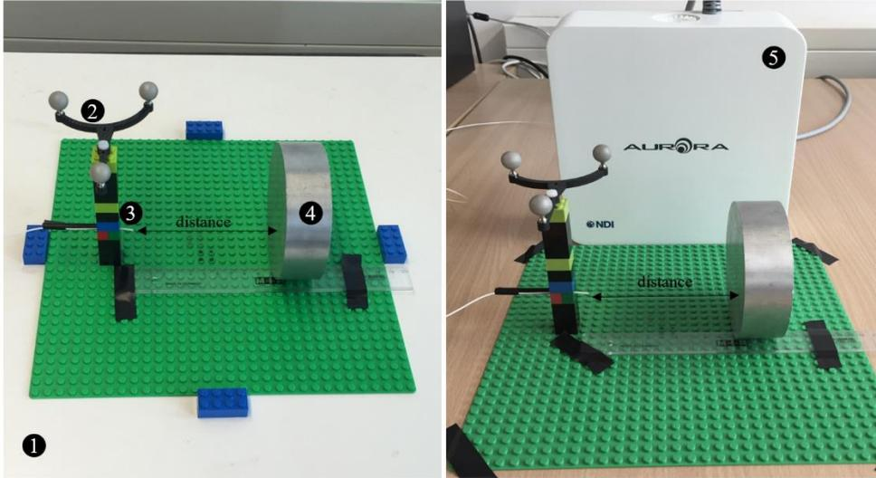
Fig. 9. Measurement of sensor pose error due to a nearby conductive distorter at different distance from 10 cm to 1 cm to the sensor coil: (1) field generator of the experimental setup, (2) optical marker with fixed pose to the sensor coil, (3) sensor coil, (4) conductive distorter, and (5) field generator of NDI Aurora system.
