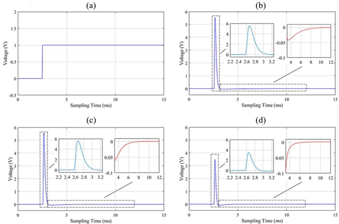
Fig. 11. The measured voltage due to a unit step excitation for distinct conductive distortions: (a) unit step excitation, (b) system response to an aluminum disk, (c) system response to a brass disk, and (d) system response to a neurological reflex hammer.
