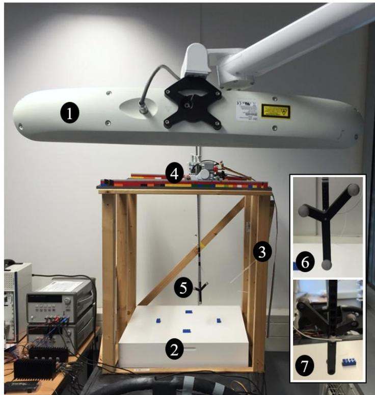
Fig. 8. Sensor pose accuracy assessment: (1) optical tracking system, (2) EM field generator, (3) test volume defined by a wooden structure, (4) LEGO robot being used to move the tracker in the 3D test volume, (5) optical marker/EM sensor with fixed locations: (6) front view—optical markers, (7) back view—rigidly fixed EM sensor.
