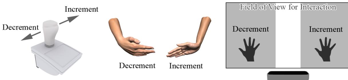
Fig. 2: Comparison of interaction with joystick (left), Myo (center) and LMC with field of view (right). The joystick is moved to the left and right to display, e.g., the next or previous image, respectively. The same applies to the hand gestures of the Myo and the hand positions in defined areas in the field of view of the LMC.
