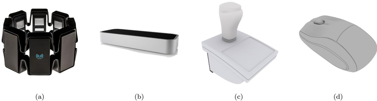
Fig. 1: Utilized input modalities of our user studies. (a) Myo gesture control armband (based on myoelectric signals of the forearm), (b) Leap Motion Controller (camera-based), (c) joystick control panel of an interventional angiography system, and (d) simple computer mouse of a workstation.
