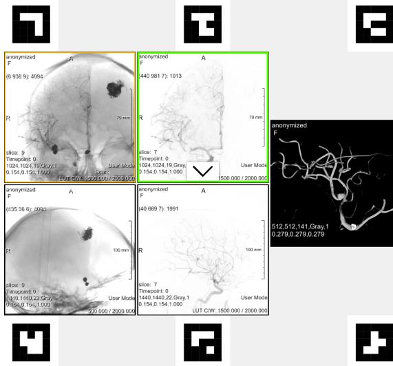
**Figure 2: Prototypical GUI consisting of four viewports showing medical image stacks (left and center) and one 3D-viewport (right). Borders indicate the currently selected viewport (green) and the gazed-at viewport (orange). Image manipulation was indicated by little arrows at the viewport edges.**
