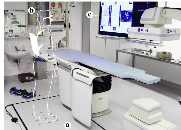
Figure 1: Technical setup for hands-free interaction consisting of a tactile floor (a), a mobile eye tracking device (b) and the large screen of an angiography suite (c).
